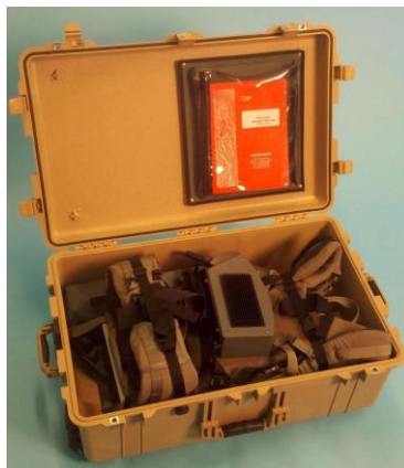
G-859SX and GPS Re-Usable Shipping Case with foam padding and transport wheels
